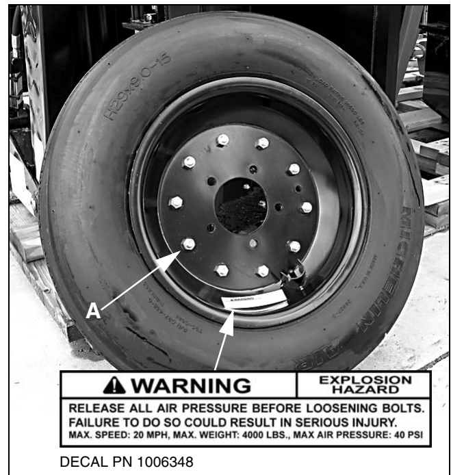
Figure 32. Split Rim Tire Servicing
